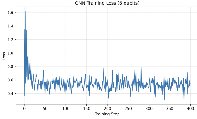
Fig. 4. Training loss for the 6-qubit QNN, showing increased oscillations and sensitivity to parameter updates.
