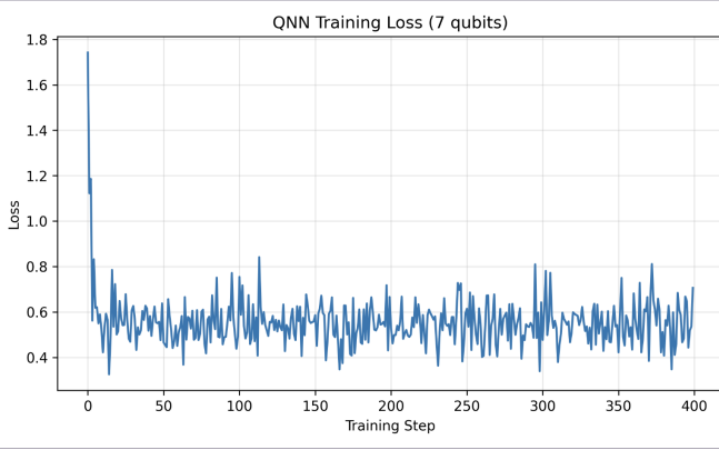
Fig. 5. Training loss for the 7-qubit QNN, illustrating reduced convergence reliability under aggressive qubit scaling.
